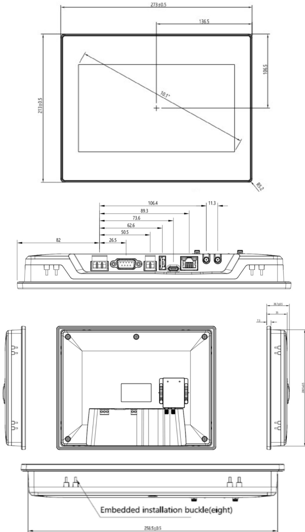
Flush-mounted installation cutout dimensions:  $260\text{mm} \times 202\text{mm} (+1.5\text{mm}/-0.0\text{mm})$
